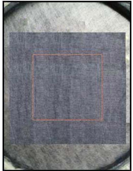
Once completed, then allow the embroidery design to stitch out (usually second and for some of the designs, the third color stop as well). Select color(s) for your design, placing the same thread in the needle as well as within the bobbin.
